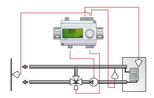
For this control mode you need two sensors, GT1 "Supply temperature" on AI1 and GT2 "Outdoor sensor" on AI2.
