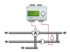
For this control mode you need a single sensor, "Supply water temperature" on AI1.
