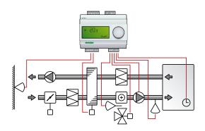
For control mode "Supply air temperature control" you need only one sensor, "Supply air sensor" on AI1.
