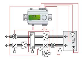
For control mode 3, "Cascade connected room/extract air temperature control" you also need two sensors, "Supply air sensor" on AI1 and either "Room sensor" or "Extract sensor" on AI2.
