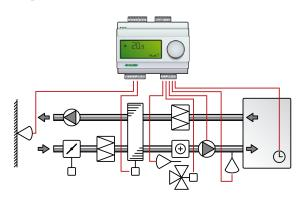
For control mode "Supply air temperature control with outdoor compensation" you need two sensors, "Supply air sensor" on AI1 and "Outdoor sensor" on AI2.
